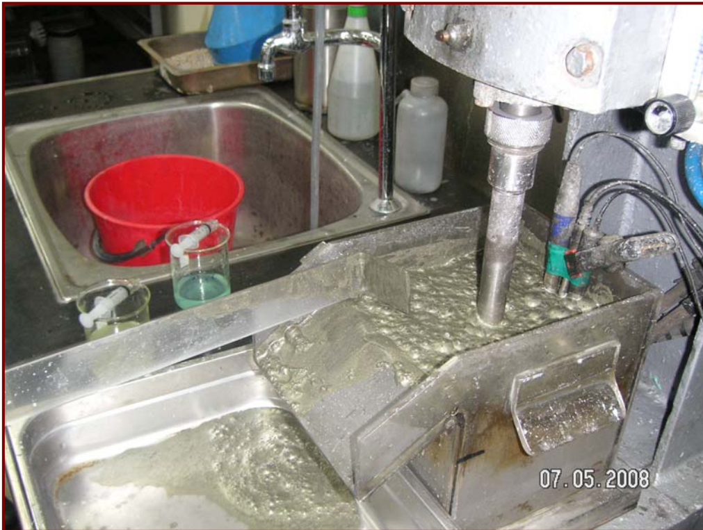
Figure 3: Sulphide flotation testwork - concentrate for 106 \mu m grind
