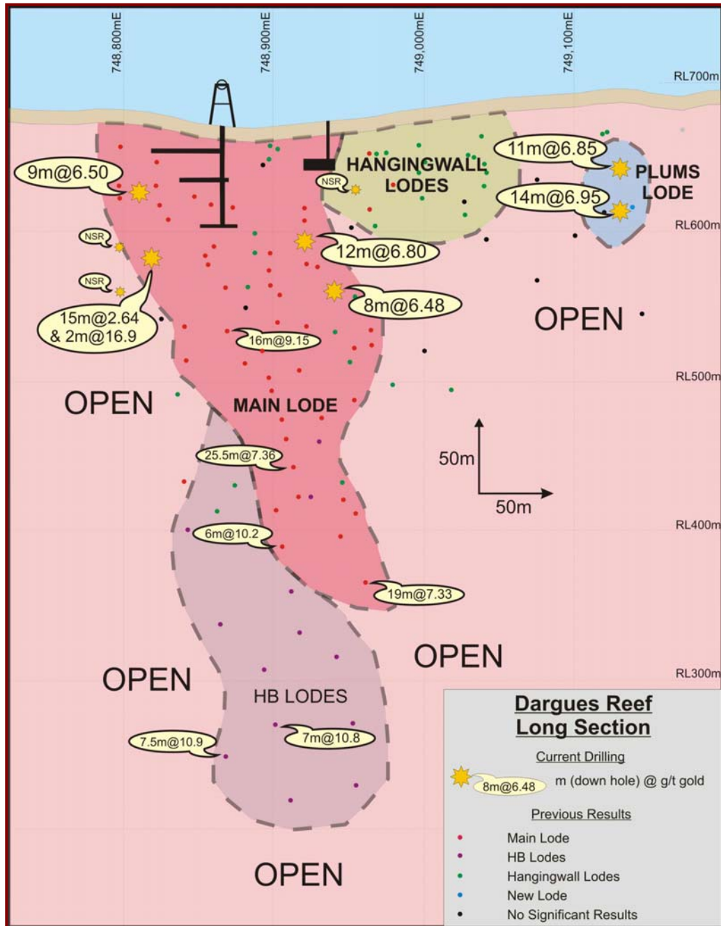
Figure 1: Dargues Reef long-section highlighting latest drilling results
