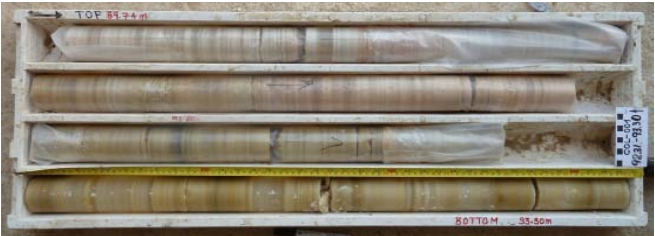
Figure 3 – COL-001 drill core showing base of strong carnallite mineralisation zone from 89.74 – 93.20m. Carnallite cores are heat sealed in plastic to prevent the core from dissolving in air.
