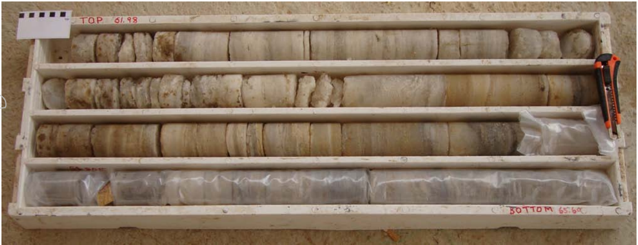
Figure 2 – COL-001 drill core showing rock salt and sylvite mineralisation from 61.98m – 65.20m.
