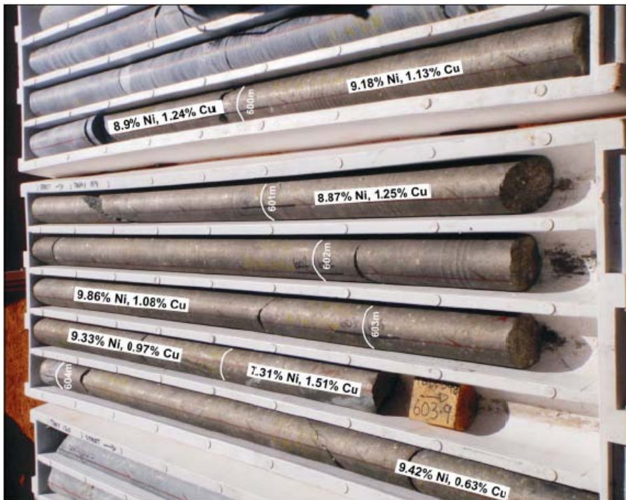
Figure 12 – JV Rosie Prospect - TBDD098 Massive Sulphide Intercept - 5.20m @ 9.13% Ni, 1.09% Cu, 0.21% Co and 7.09g/t PGEs (PGEs include 2.22g/t Pt, 1.74g/t Pd, 0.82g/t Rh, 1.79g/t Ru)
