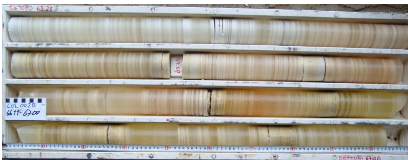
Figure 5 – COL-002B drill core showing the base of a strong carnallite mineralisation zone from 63.25m – 67.00m.
