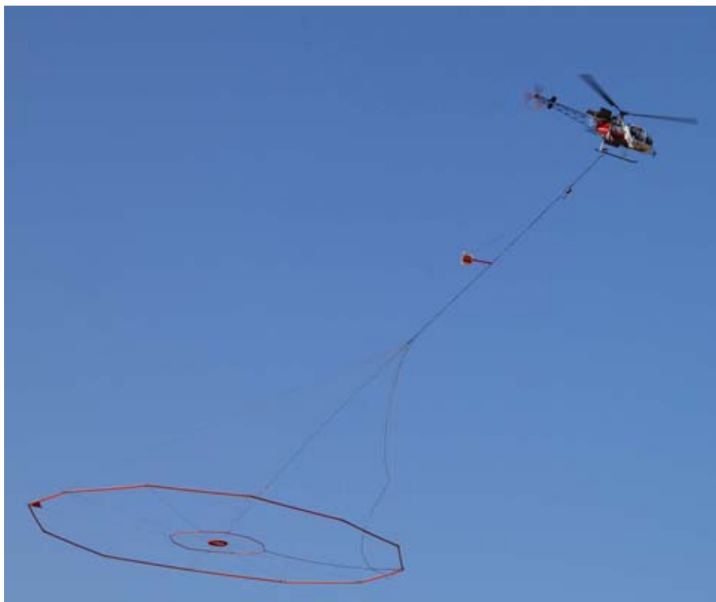
Figure 4: Aerospatiale Lama helicopter with Geotech VTEM and magnetic systems suspended beneath
