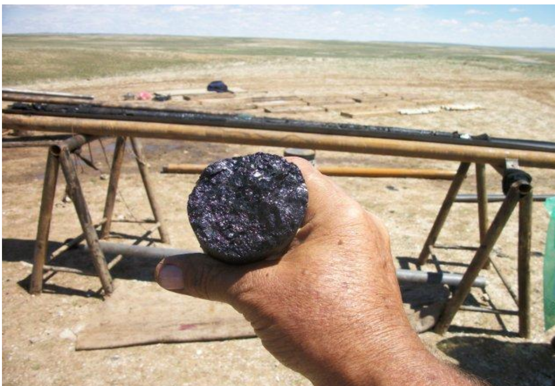
Core sample from BTE-2 indicates good levels of vitrinite.
