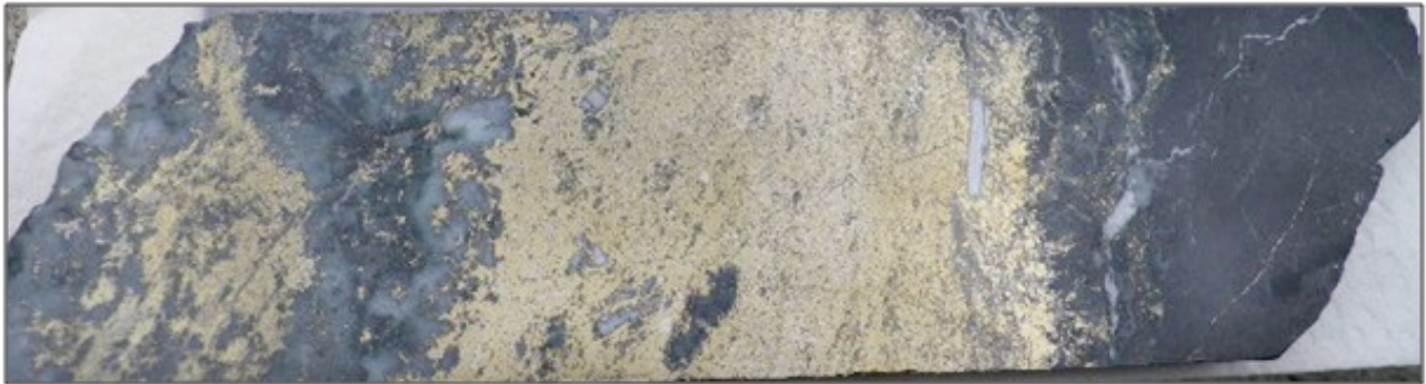
Massive copper mineralisation (as chalcopyrite) at 177.6m in hole H99-4.
