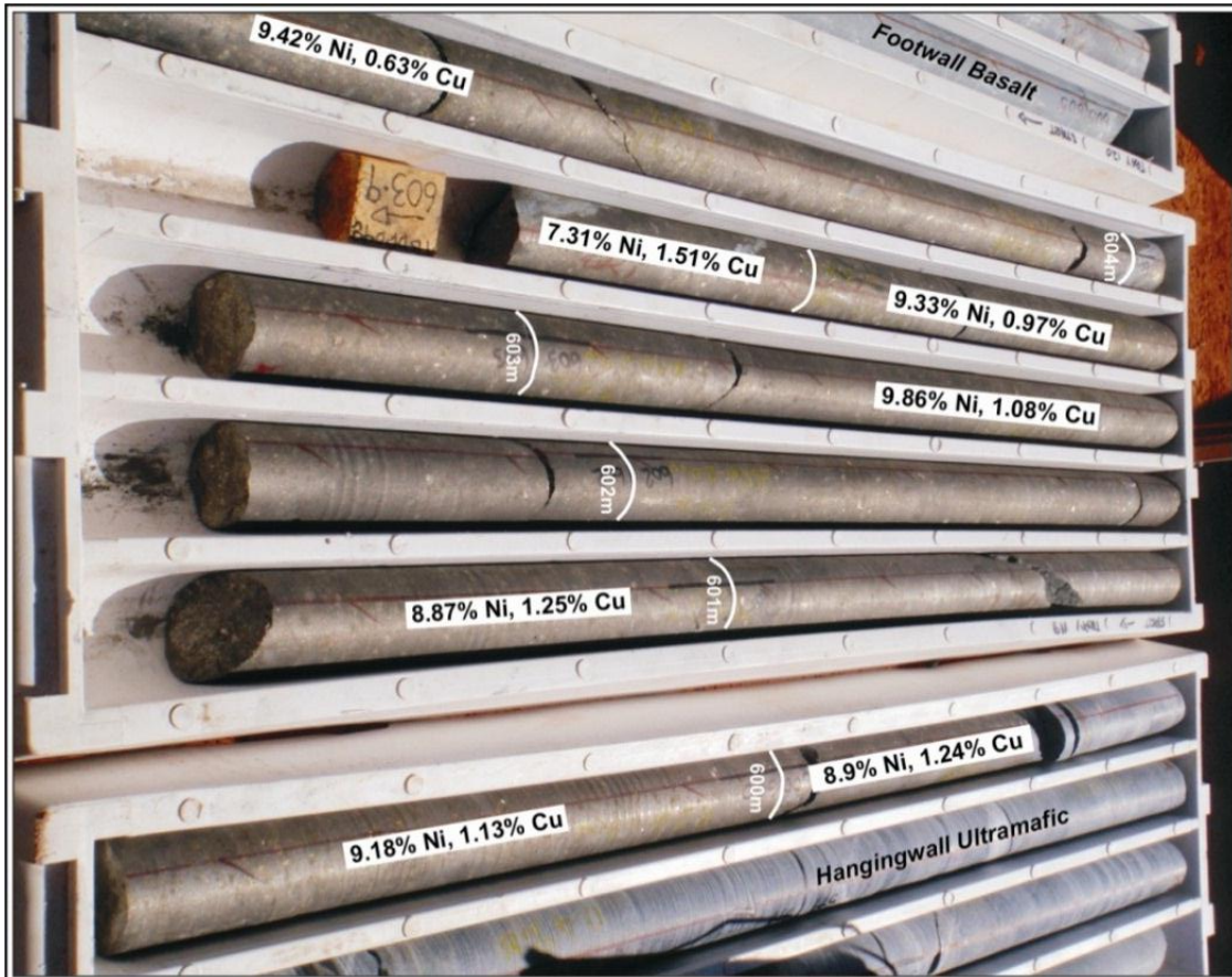
Figure 4: Rosie deposit massive sulphides in TBDD098, with coarse grained pentlandite porphyroblasts.
