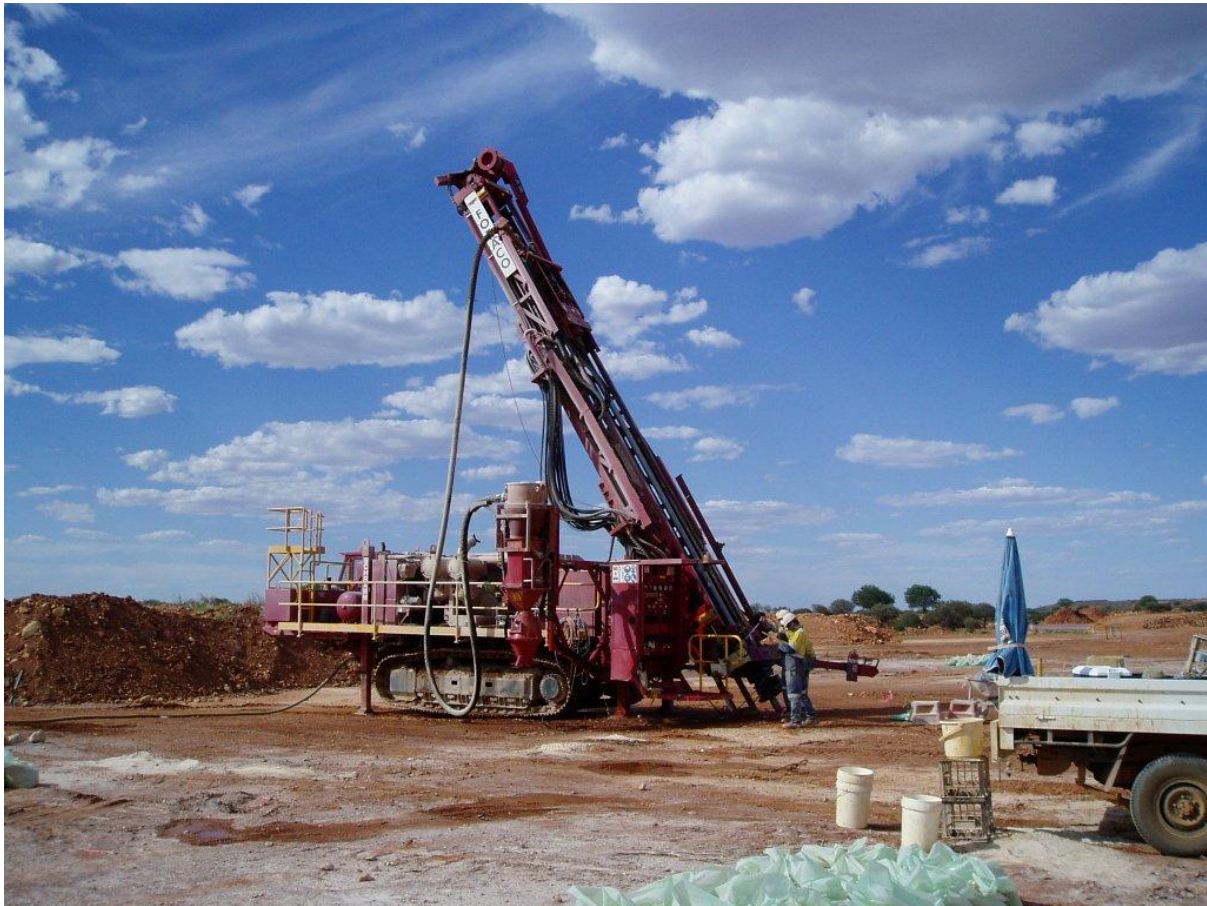
Figure 1 Air-core drilling adjacent to Reward Pit, Burnakura
