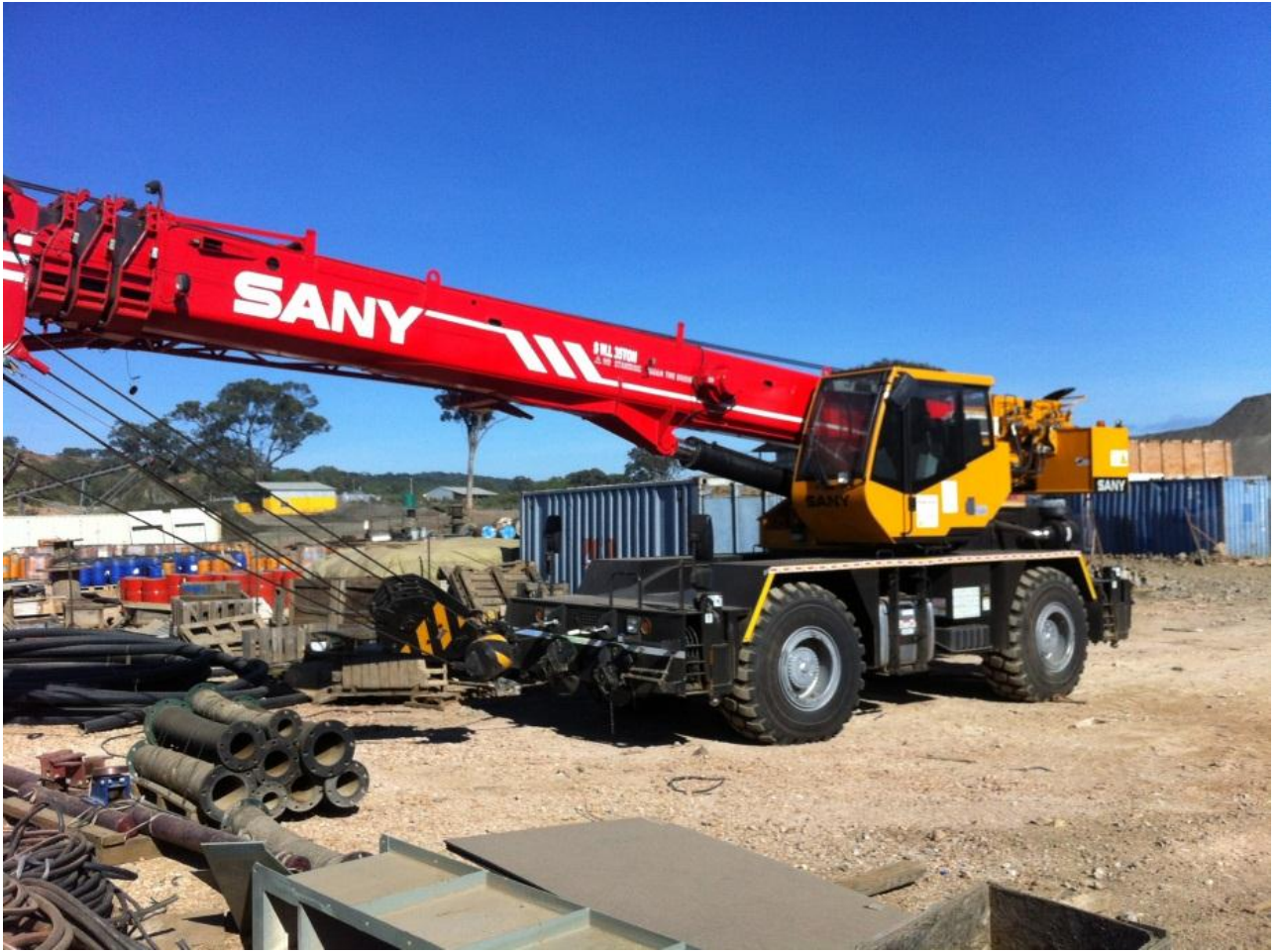
The 35t crane for the erection of the SXEW plant at the Kipoi bonded customs clearing facility
