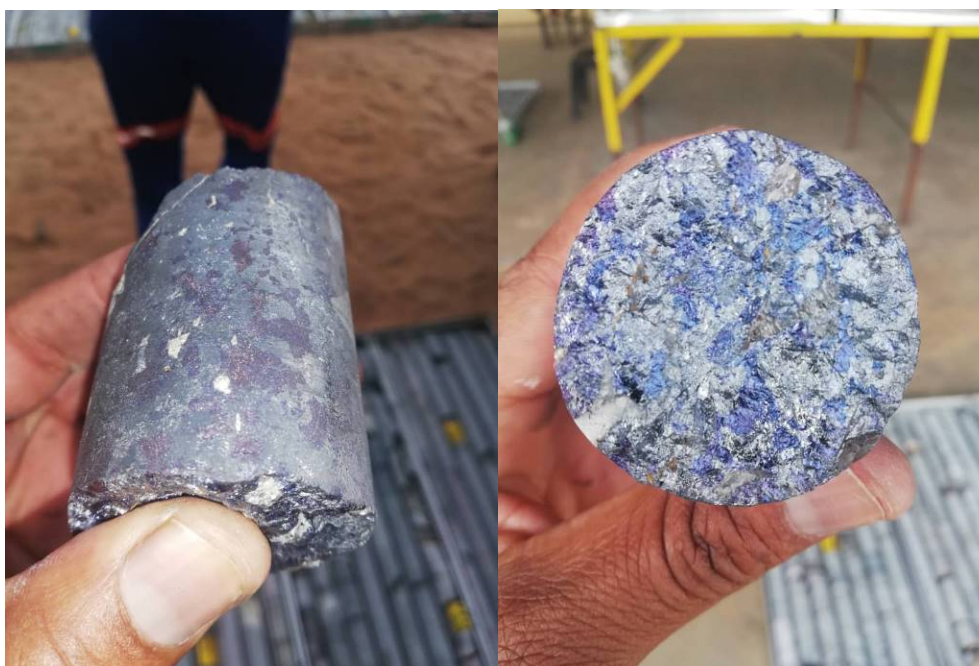
Figure 5: Massive bornite-covellite-chalcocite copper sulphides in hole MO-A4-029D within a 1m vein interval from 130.14m down-hole depth. Assays are awaited for MO-A4-029D to confirm the copper grade in this interval.
