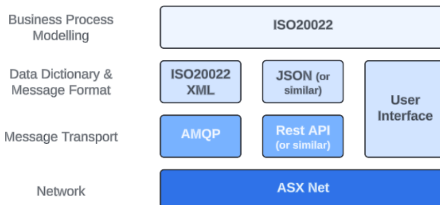
Diagram 2.0: Proposed data access interfaces
